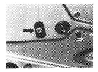
10 Adjust lower lift limitation with the stop at the window lifting rail so that the upper edge of the window glass is flush with the sealing rails.
