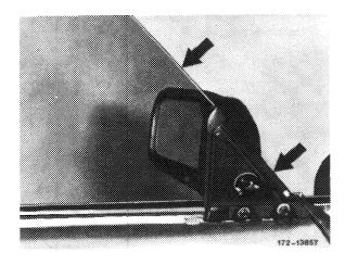
**Note:** A correction can be made by moving the rear screw at the window lifter and by the front stop angle for the upper lift limitation.
