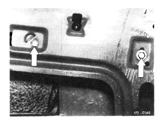
3 Loosen rear window lift rail screw.
