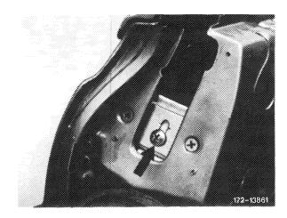
**Note:** Upon subsequent fitting of the rear quarter window, the front edge of the rear quarter window must be adjusted parallel to the rear edge of the crank window.
