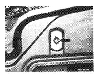
If required, the tilt of the crank window can additionally be corrected after loosening the three screws at the window lifting rail.
