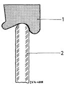
8 Adjust rear guide rail in the elongated hole so that the rear edge of the crank window contacts the sealing rubber of the rear quarter window along the entire length with the door closed.
