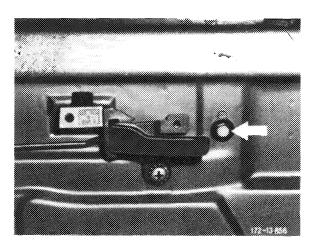
4 Loosen screw for upper stop angle at the rear.
