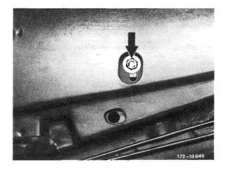
5 Remove lower nut at the rear window guide rail.
