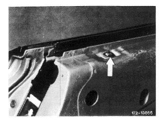
8 Remove both screws at the rear guide wedge and remove guide wedge.
