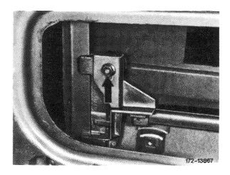
4 Remove stop angle for top lift limitation at the rear.
