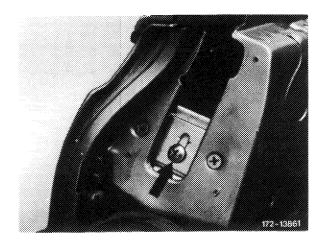
9 Lift crank window and pull rearwards out of the door.
