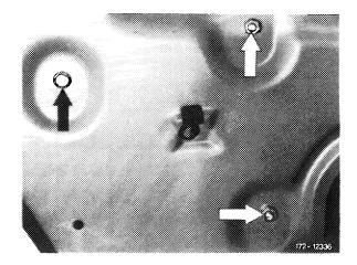
10 Press window running rail forward and remove window lift with motor downward.
