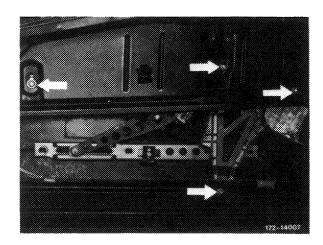
8 Remove window lifter with motor at the bottom.
