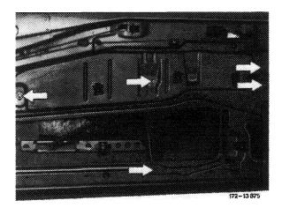
6 Remove window lifter via access opening.
