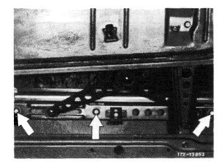
5 Unscrew screws at door inner panel.
