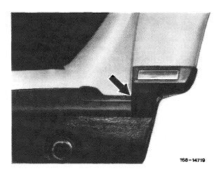
7 Attach trimstrip to door at front slot and push completely forward. Then push trimstrip in range of slot against door and pull toward the rear, so that the rear portion of the fastening hook engages in door.
