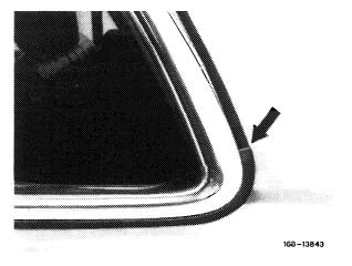
3 Starting at the rear, knock cover onto the weatherstrip by means of the caulking tool.
