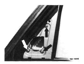
4 Lift ornamental rod with a plastic wedge starting at one side and pull it out of clips.
