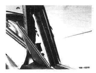
3 Remove screws and take off outer plate.
