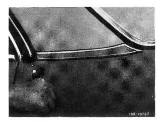
2 Insert plastic wedge or similar in bulge and press cover out of clips.
