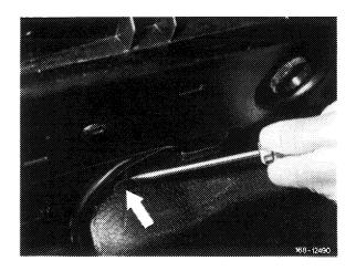
2 Press out rivet lower section with a screwdriver.
