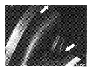
7 Tilt cover inward into trunk and remove.
