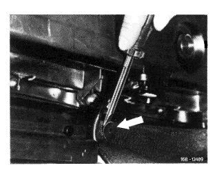
3 Remove front metal screw (only applicable to first models).
