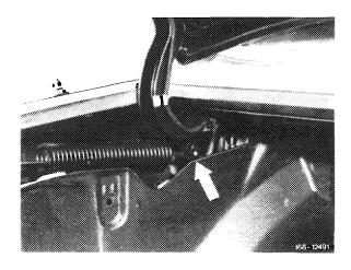
6 Pull cover out of partition, starting at top and then bottom.
