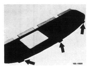
**Note:** Make sure that three retaining cams of hat rack are slid underneath the metal holders provided.
