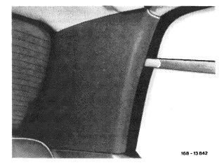
2 Pull trim panel front rearwards towards the center of the vehicle and out of the two clips.
