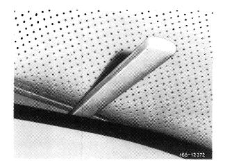
2 Press the three plastic hooks out of holder from the outside with a plastic wedge.
