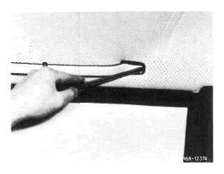
3 Pry off edge guard strip in area of headliner with a plastic wedge.
