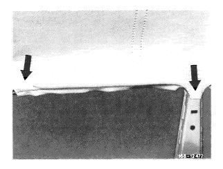
17 Glue headliner to rear pillar and rear window opening at corners of seam. Cut off protruding headliner material.
