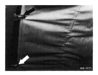
14 Stretch headliner and glue it to rear window opening at center area of seam (MB-PVC glue, Part no. 001 989 30 71).
