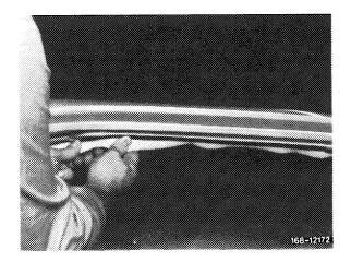
16 Stretch headliner and glue it to center pillar and front roof frame.
