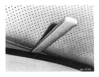
4 Remove both lower screws from center pillar trim and pull down center pillar trim.
