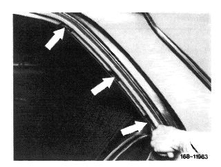
7 Detach headliner at side roof seam.
