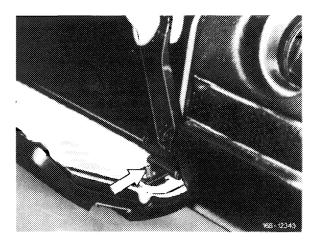
8 Lift inner stop bracket with glove compartment lid upper section out of instrument panel.
