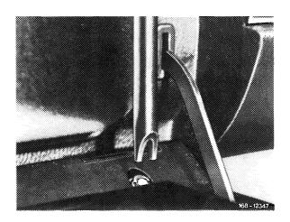
3 Position outer side retaining pin upright.
