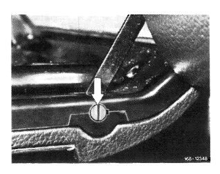
4 Pull side pin out of glove compartment lid.
