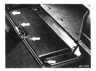
2 Remove both slotted nuts, using a standard slotted nut wrench.
