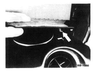
3 Tilt cover forward, so that the cam can be pulled out of opening in instrument panel.
