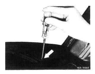
2 Lift cover a little and swing toward center of car just enough, that the side hook disengages at the instrument panel.
