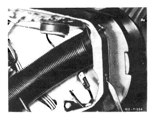
11 Detach connecting lever (arrow) for fresh air flap and pull off connecting hose between heater box and both center fresh air nozzles.
