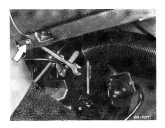
13 Unscrew left and right bolts underneath instrument panel.
