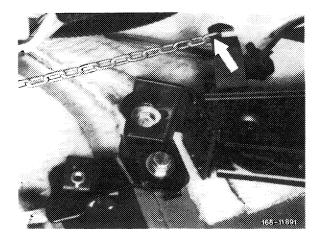
10 Pull air hoses off of left and right side ring nozzles.
