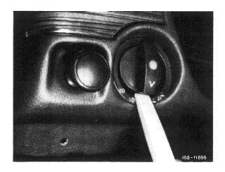
8 Unscrew nut on rotary light switch (wrench size 24 mm).
