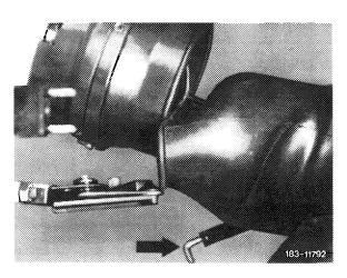
12 Unscrew bolt on support, counterholding nut.
