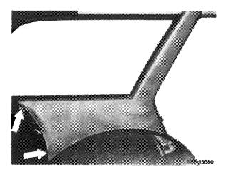
5 Push rubber frame of quarter window from inside over groove by means of a plastic wedge and remove glass in upward direction.
