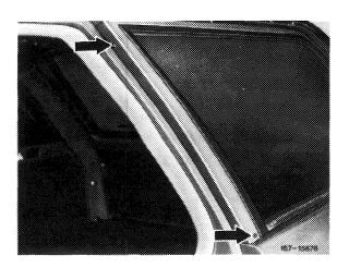
3 Remove paneling on rear roof frame (68-447).
