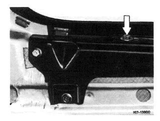
17 Adjust lateral contact pressure of the rear quarter window glass with the screw (arrow).
