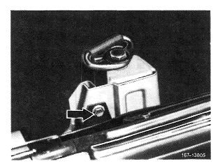
5 Remove lock at intermediate lever from window lifter and disconnect intermediate lever at the guide plate.
