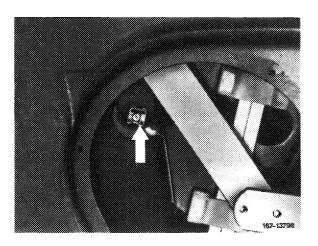
6 Unscrew both screws at the top of the guide plate.
