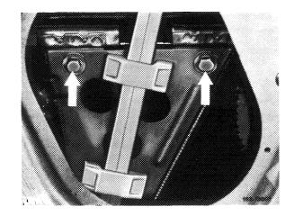
7 Unscrew both screws at the front of the guide rail and pull out guide rail downwards from the guide jaws of the rear quarter window.
