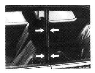
16 Adjust stop for upper lift limitation with the screw (arrow) at the shell cover.
