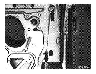
8 Lift quarter window glass forward and out of the shell.
