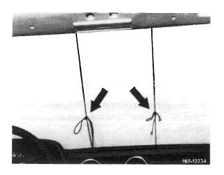
16 Apply light pressure against windshield, while a helper on the inside of car lifts the lip of the rubber frame over the spot welded flange of the window opening by carefully pulling out the cord, starting at the bottom.
