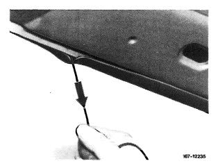
17 Pull outer rubber lip in outward direction by pulling out the additionally inserted cord in area of front wall pillar.
