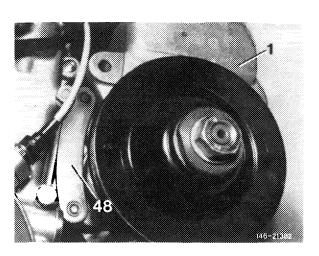
24 Unscrew hex. nut from drive shaft and pull off pulley by means of puller.
