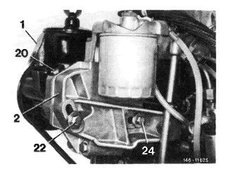
10 Remove powersteering pump while paying attention to tensioning piece (21).
