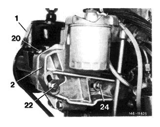
28 Attach power steering pump with hex. bolt (23) to carrier (do not forget 5 mm washer), but do not yet tighten hex. nuts.
