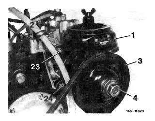
29 Mount V-belt and tension with hex. screw (20). Then tighten all hex. bolts and hex. nuts.
