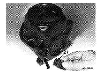
27 Insert power steering pump into carrier, screw hex. screw (20) into clamping piece. Attach pump with hex. bolts (22) and (24), but do not yet tighten hex. nuts.
