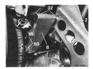
36 Attach pump in holder (8) or carrier with hex. screw (36), but do not yet tighten.
