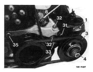
31 Screw hex. nut on gear wheel (27), mount V-belt and tension belt with gear wheel. Then tighten all hex. nuts and bolts.
