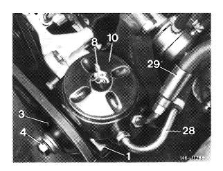
6 Loosen hex nut (4) on input shaft while holding pulley and flat profile.
