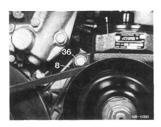
37 Screw hex nuts on gear wheel (25). Place V-belt on pulley. Tension pulley with gear wheel. Tighten hex. bolt and hex. nut on gear wheel.
