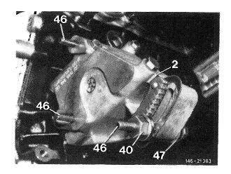
39 Insert power steering pump in mounting bracket, screw both hex. head screws into holder (48).
