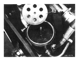
5 Loosen high-pressure expanding hose (29) and elbow (28) for return hose on powersteering pump.
