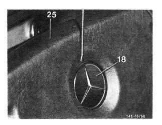
4 With steering lock (10) engaged, unscrew countersunk screw from steering wheel shaft.
