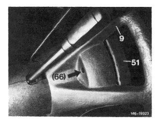
5 Lift complete airbag unit (51) from steering wheel.
