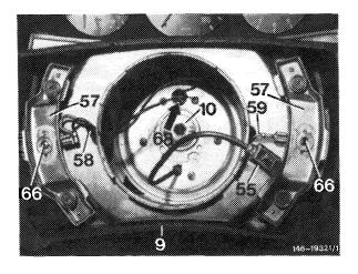
16 Connect cable (68) on plug connection of slip ring.
