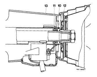
9 Attach pad to horn carrier. Unbuttoning of pad is done best by starting at a corner near steering wheel spokes. Do not use force so that the horn carrier is not damaged.
