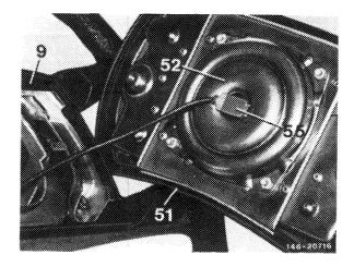
7 Remove airbag unit from steering wheel.
