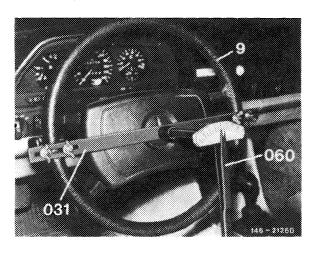
5 The steering must be readjusted, if no increase of friction torque shows up in center range when turning steering from lock to lock.
