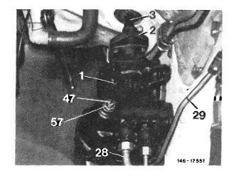
7 Check friction torque. In center range, torque should be 30–60 Ncm above basic friction torque measured before.
