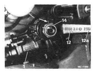
2 Pull pitman arm (12) from pitman shaft with puller (065).
