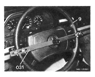
4 Insert torque wrench (060) into mounting (031) and turn steering several times from lock to lock, while measuring friction torque.
