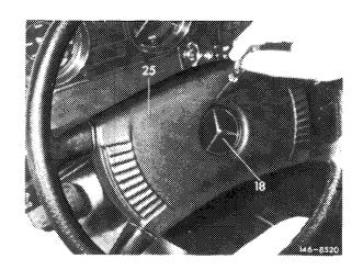
3 Position torque wrench on hex. nut of steering shaft, measure the force required for turning steering shaft which should not exceed 5–7 Nm.
