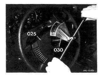
4 Insert company symbol into pad or attach pad to horn bracket of steering wheel. Start by unbuttoning pad in range of steering wheel spokes. Do not use force, so that the horn bracket is not damaged.
