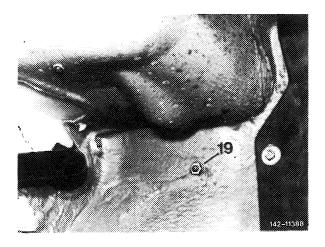
3 Unscrew hex. nut (19) in engine compartment at front end.
