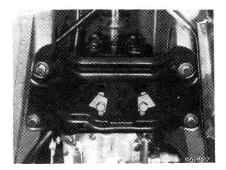
Rear engine carrier on all 5- and 6-cylinder engines and on 4-cylinder engines with automatic transmission.
