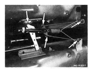
24 Tighten clamping nut on propeller shaft. Watch out for good seat of sleeve. Tightening torque of clamping nut on 2-piece propeller shaft 30—40 Nm and on 3-piece propeller shaft front 30—40 Nm, at rear 200 Nm.
