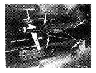
4 Loosen clamping nut of propeller shaft for approx. 2 turns without pushing back rubber sleeve (slides along).
