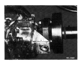
19 Attach propeller shaft intermediate bearing to frame floor, but do not yet tighten.
