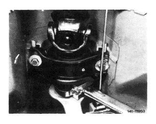
25 Tighten hex. bolts for attaching propeller shaft intermediate bearing to frame floor to 25 Nm.
