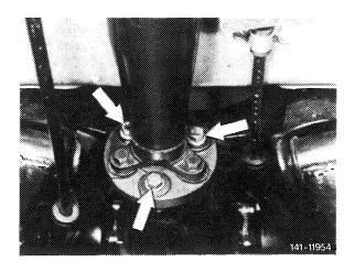
8 Unscrew hex bolts for attaching propeller shaft intermediate bearing to frame floor.
