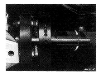
10 On vehicles up to July 1982 with 5-cylinder Diesel engine, as well as with engine 102, mark front and rear propeller shaft with vibration eliminator in relation to each other (refer to arrows). Remove front propeller shaft in forward direction and rear propeller shaft in rearward direction.
