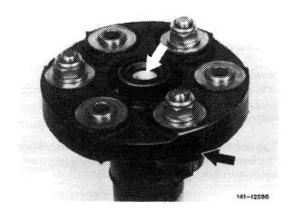
18 Push front propeller shaft with vibration eliminator from the front through the bridge and slip on centering pin on transmission. Push rear and front propeller shaft, as marked, together at clamp connection and attach to centering pin on rear axle.
