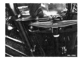
Rear engine carrier on 4-cylinder engines with manual transmission
