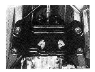
23 Attach cable controls and compensating lever of parking brake and adjust (42–525).
