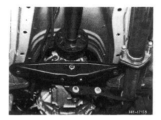
13 Check companion plates (12), centering sleeves (10) and propeller shaft intermediate bearing for damage, replace damaged components.
