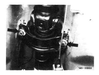
9 Force propeller shaft from centering pin of rear axle. Pull out propeller shaft without vibration eliminator toward the rear.
