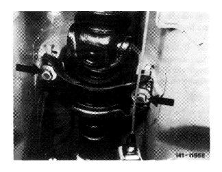
20 Flange propeller shaft to transmission and to rear axle. Tightening torque of self-locking hex nut 45 Nm.
