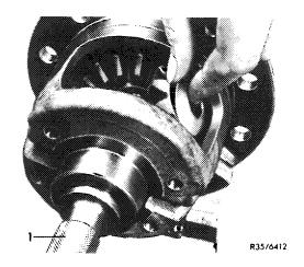
16 Insert assembly mandrel (3) instead of differential pinion shaft to locate differential pinions and ball washers.
