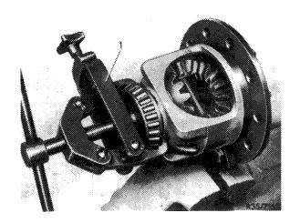
3 Knock clamping sleeve (28) for differential pinion shaft (36) out of differential housing (31) by means of a matching mandrel.
