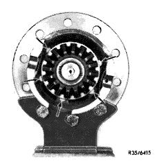
13 Install righthand side gear with friction discs and assembly mandrel.
