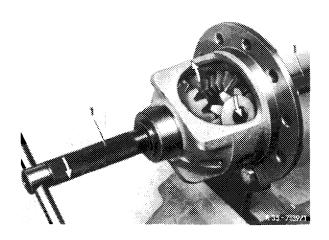
11 Slip assembly mandrel (2) instead of differential bolt into differential housing to locate differential pinions and ball washers.
