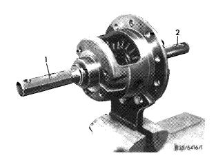
6 Turn out differential pinions with ball washers and remove.
