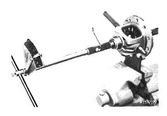
13 Knock in differential bolt while paying attention to bore for clamping sleeve.
