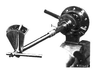
18 Knock in differential pinion shaft and remove assembly mandrel (3).
