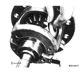
7 Remove righthand side gear with friction discs.
