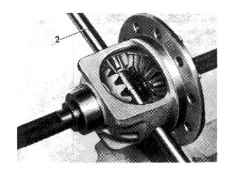
12 Check friction torque. Friction torque should amount to 30–90 Nm, at restraining points up to 100 Nm.
