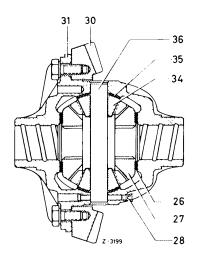
4 Force out differential pinion shaft and remove differential pinions, side gears, thrust washers and ball washers.
