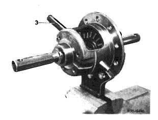
17 Check friction torque. Friction torque should amount to approx 80–140 Nm.
