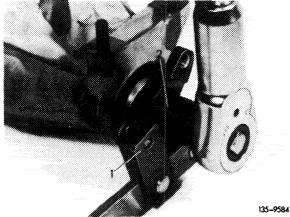
16 Pull universal flange from drive pinion with puller, if required.
