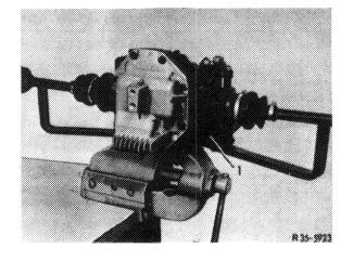
3 Unscrew end cover (4) from rear axle housing.
