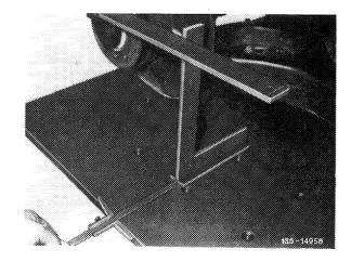
10 Place try square at the rear against inner mark of straightedge using a second try square for this purpose.
