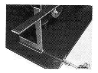
12 To find toe-in per wheel (VSR1) determine difference between values measured at the front and rear and enter into data sheet.
