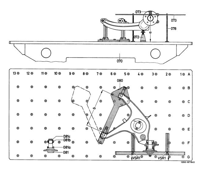
Height adjusting dimension for rear axle shaft flange at upper edge for wheel fit
