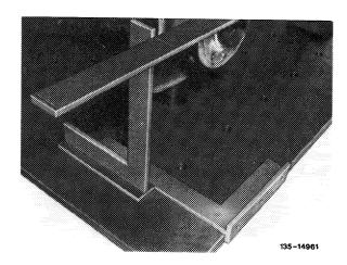
11 Measure rear distance from edge of measuring table to try square or to straightedge with depth gauge and write down value.
