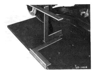
9 Measure front distance from edge of measuring table to try square or to straightedge by means of depth gauge and write down value.
