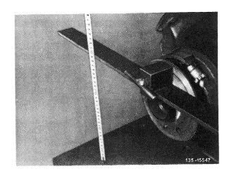
8 Position try square at front against inner mark of straightedge, using a second try square for this purpose.
