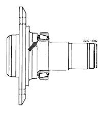
21 Press inner race (16) of outside tapered roller bearing on rear axle shaft flange (15).
