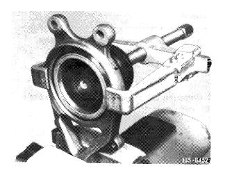
10 Unlock slot nut on rear axle shaft flange and unscrew.
