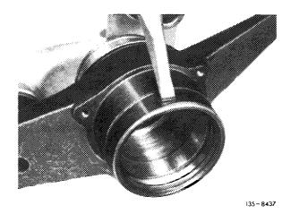
16 Pull outer race of outside tapered roller bearing from wheel carrier.
