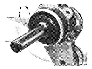
19 Check rear axle shaft flange for vertical and lateral runout.
