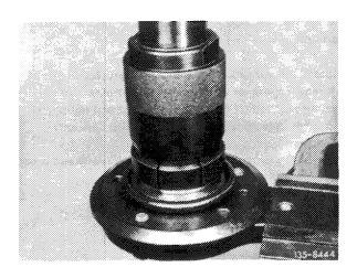
15 Knock outer radial sealing ring from wheel carrier.
