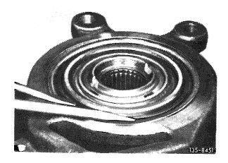
8 Pull caliper carrier with radial ball bearing from wheel carrier.
