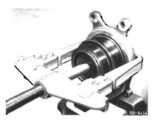
23 Press caliper carrier with radial ball bearing on wheel carrier by means of installer (01).
