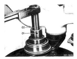
11 Remove sealing ring and push off radial sealing ring uniformly by means of a screwdriver.
