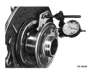
34 Adjust end play (0.04-0.06 mm) of rear axle shaft flange by tightening slot nut. Turn rear axle shaft flange several times and check end play at several points.
