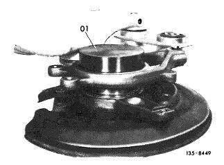
24 Mount protective ring and secure with locking ring.
