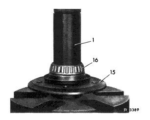
22 Press radial ball bearing into caliper carrier with remover and installer up to stop and secure with locking ring.
