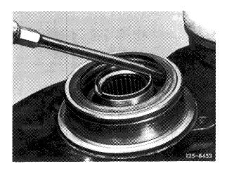
12 Push wheel carrier from rear axle shaft flange by means of two-arm puller and thrust piece (01). Remove wheel carrier with coupled semi-trailing arm and inner race of inside tapered roller bearing.
