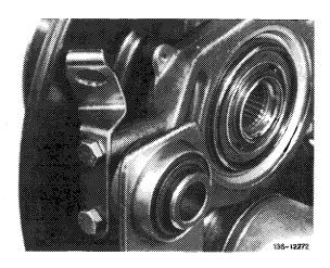
26 Install outer races of both tapered roller bearings into wheel carrier by means of installer (01).
