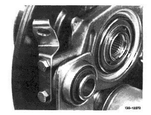
7 Remove locking ring and remove together with protective ring.
