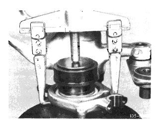
9 Remove locking ring and push radial ball bearing out of caliper carrier.
