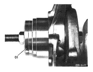
27 Coat seat for outer radial sealing ring on wheel carrier with sealing compound and carefully mount new radial sealing ring by means of installer (01) in such a manner that ring rests against shoulder of wheel carrier.
