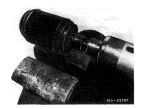
3 Plug thrust piece (012g) and holding ring (012h) on control arm (4). Place puller (019) on tool and screw-in bolt until axial- and radial-torsion rubber bearing is pushed out of control arm.
