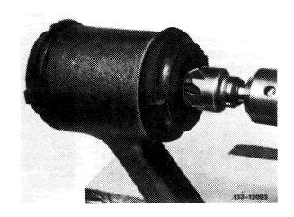
4 Loosen rubber bearing by moving bearing back and forth in control arm and remove.
