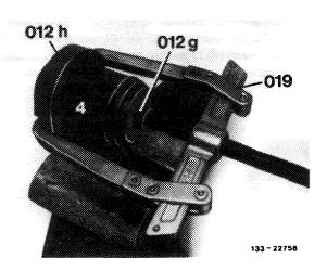
4 Knock second, remaining axial-torsion rubber bearing (16) out of control arm (4) by means of a punch.
