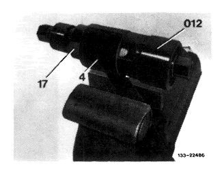
Note: Make sure that the two flats of the rubber bearing are in line with reference flat of control arm.
