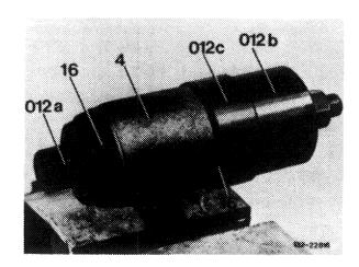
11 Check seat of mounted axial-torsion bearing (16). Both bearings should rest against control arm (4).
