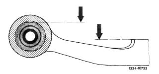
8 Insert radial-torsion bearing (17) until rubber edge is flush with edge of control arm with radial-torsion bearing relaxed.
