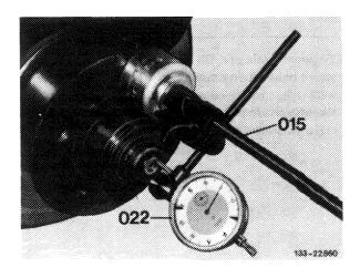
7 Check end play of wheel hub by pulling and pushing on flange.
