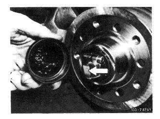
5 Loosen hex socket screw of clamping nut (9d) and tighten clamping nut while simultaneously rotating hub (9) in such a manner that the hub can be turned with considerable effort only. Then screw clamping nut back for approx 1/3 turn and release tension by applying a blow with a plastic hammer against wheel spindle (5a).
