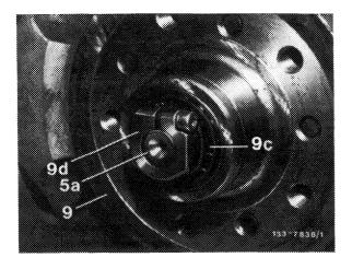
6 Place test instrument (015) on front wheel hub and set dial gauge (022) to approx. 2 mm preload.
