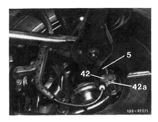
7 Unscrew hex bolts (refer to arrows) for attaching brake support to frame floor.
