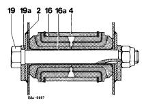
Bearing of lower control arm on frame cross member (3-part bearing)
