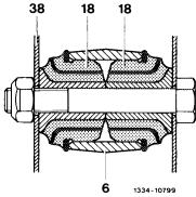
Support of upper control arm on torsion bar
