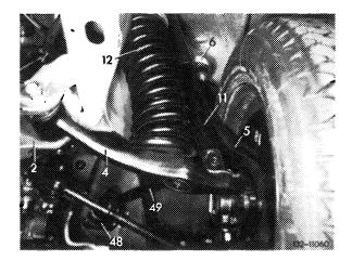
25 Place eccentric bolt (19) of camber adjustment to previously made mark and tighten.
