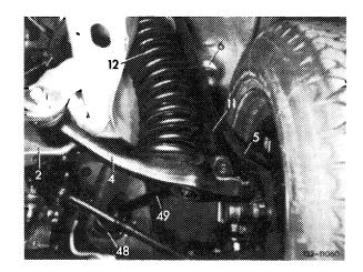
4 Loosen ball joint of track rod (28) on steering knuckle arm (29) and remove with tool (040).
