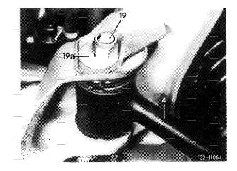
11 Remove support of upper control arm on torsion bar.
