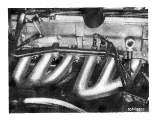
3 Mount exhaust manifold with new gaskets. Make sure that the bead (arrow) points toward exhaust manifold.
