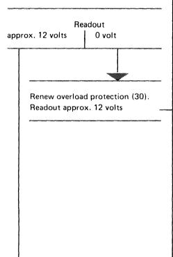
Attach relay for voltage supply (29) to plug in such a manner that voltage on jack 3 can be measured with plus (positive) cable of voltmeter.
