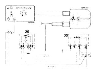
Attach overload protection (30) to plug in such a manner that the voltage on terminal 6 can be measured with plus (positive) cable of voltmeter.
