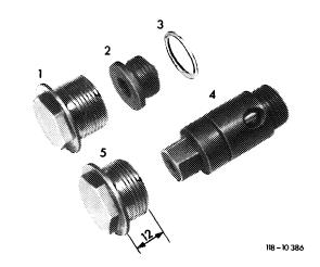
For subsequent installation of a 5 bar pressure relief valve into the following vehicle models, connect line of fuel evaporation control system to cylinder head (arrow):
