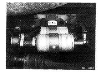
8 Clean fuel pump and fuel filter externally and mount in addition to plastic sleeve (slip up to bead of pump).
