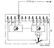
Fuel pump relay Refrigerant compressor
