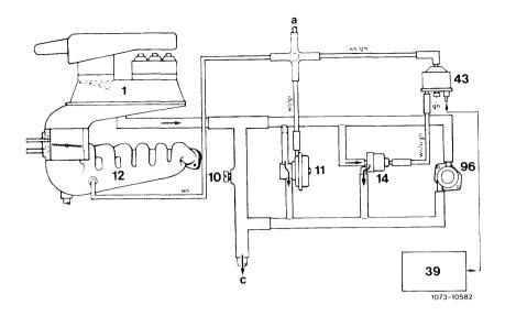
Function diagram idle speed stabilization on engines with refrigerant compressor 1 Mixture controller 43 Switchover valve rpm increase
