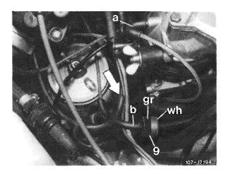
Stop engine, pull off fuel pump relay (arrow).
