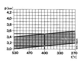
Note: Starting model year J 1981, USA 1980 the vacuum flow is straight. Control pressure is therefore independent of intake manifold vacuum.
