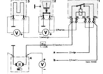
Mixture controller with safety switch
