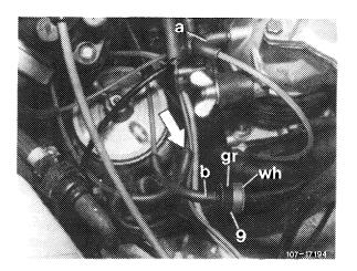
Plug vacuum pump to vacuum line toward warm-up compensator and activate warm-up compensator with 0.5 bar vacuum.
