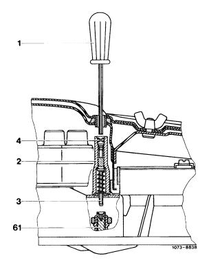
Release screw driver, compression spring will push adjusting device out of mixture control screw.
