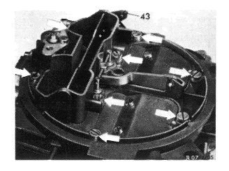
5 Force off carburetor cover at forcing-off point and remove.
