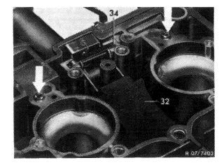
Tighten carburetor fastening nuts uniformly and crosswise to specified torque.
