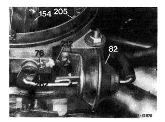
**Note:** If the adjusting pin (212) has been automatically released, or if the restoring spring must be replaced, install a modified adjusting pin, which is knurled at contact surface of locking screw (76).
