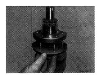
4 Introduce crankshaft into a suitable steel tube (approx. 165 mm dia. x 420 mm long) and place self-made rivet support (2) underneath.
