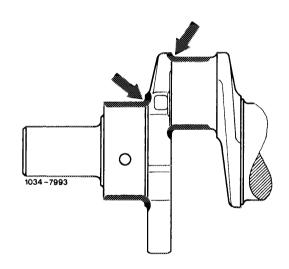
When hardening journals without hardened fillets, maintain distance A between runout of hardened surface and fillet (4–5 mm).
