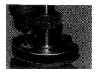
3 Slip-on new or former, undamaged additional weight together with 4 countersunk rivets.
