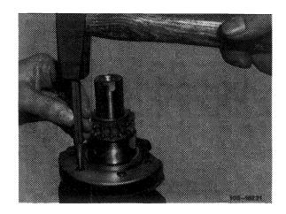
2 Drill into rivet heads with a 6.5 mm dia. drill and knock out.
