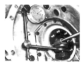
6 Rotate crankshaft for one full turn by means of tool combination. Vertical runout should not exceed max 0.10 mm.
