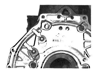
For cleaning main oil ducts during engine repairs, the steel balls must be knocked-out from direction of front end of engine.
