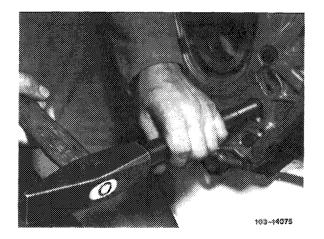
If the mandrel has no stop, do not exceed dimension a = max. 3 mm to prevent cracking of crankcase.
