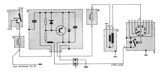
Fig. 1 Wiring diagram of transistorized coil ignition
