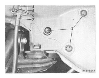
• Check the three fixing bolts for tight fit and retighten if necessary
