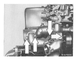
• Retighten all nuts and bolts of the intake and exhaust manifolds on the cylinder head.
