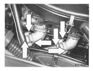
Retighten bolts of exhaust flanged connections.
