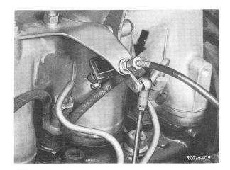
• Turn the knob on the instrument panel fully to the right. Then turn the knob back to the left; there should only be about 1/2 a revolution of free travel until an increase in idle speed is produced. Adjust with adjustment screw (arrow) if required.
