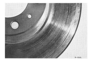
• Clean the air ducts of ventilated brake discs with a thin piece of wire, observing that the balancing clamps are not knocked out of the air ducts. Blow out the dirt loosened in this way from the ducts with compressed air.
