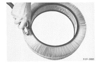
On vehicles with Engine M 130.923 (USA-Version, model year 1972) the air filter contains a ring of charcoal besides the air filter element.
