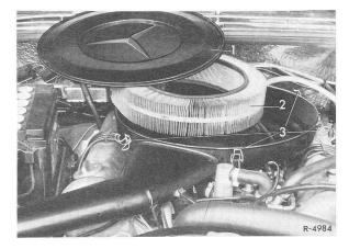
• Blow out element with compressed air from inside (max. 71 psi).
